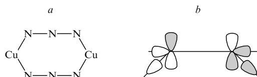
Figure 11. Structure (a) and orbital overlap scheme (b) for binuclear Cu(II) complexes with \mu_{1,3} -bridging ligands \text{N}_3^- .
