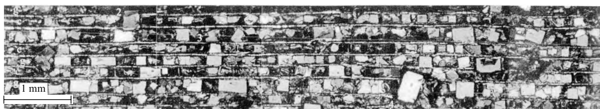
Figure 27. Biaxial texturing of superconducting phase YBa 2 Cu 3 O x on a silver substrate with artificial relief.
