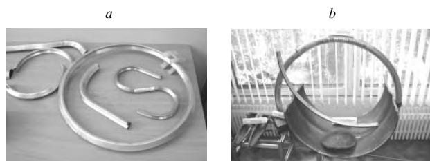
Figure 18. Detonation cutting: cumulative charges (a) and slit items (b).
