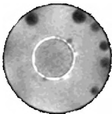
Figure 3. A 2D NMR image of a cylindrical ampoule filled with a \text{H}_2\text{O}_2 solution. A catalyst granule ( \text{Pt}/\gamma\text{-Al}_2\text{O}_3 ) is located at the centre of the ampoule.
