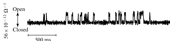
Figure 12. Conductance of the K^+ ions at 60 mV (peptide 3 , the probability of channel opening is 0.14). 11
